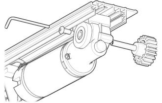
Insert the motor wheel on the opposite side of the motor and tighten the bolt using Allen key.
