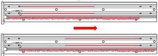
6) Place the power cable in extruded recessed area. Unit is shown upside down below.
