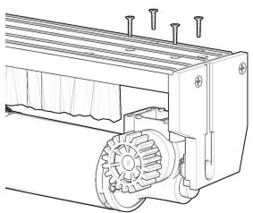
8) Reattach the control panel to the metal bars in the unit base using the Allen key. Do not tighten
