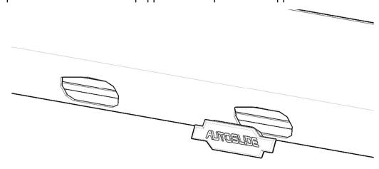
**Note**: Aligning the mode control pad to the cut in the unit cover may require some slight adjustment to the left or right of the control panel. Once aligned properly, tighten the four Allen key bolts holding the control panel in place. The unit is now re-handed and ready for install.
