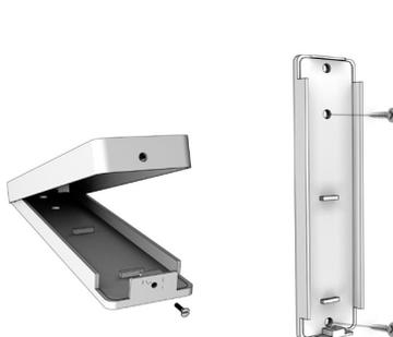
1. Undo the screw at the bottom of the switch.
