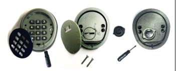
Pry open blue cover Unscrew back plate Turn cap to expose battery
